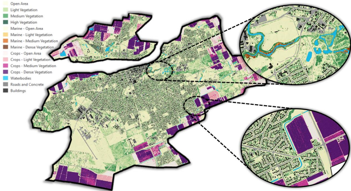
Figure 8. TUFLOW Model Hydraulic Roughness Distribution
